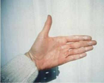
**Chalking** is caused by a degradation of the resin systems at the surface of the finish, due predominantly to ultraviolet (UV) rays. As the resin system breaks down, resin particles along with imbedded pigment particles lose adhesion and take on a white appearance, creating a chalky powdered surface. Due to both chalk and fade being directly associated with the impact of UV rays, some product manufacturers will consolidate the two into one warranty offering.
