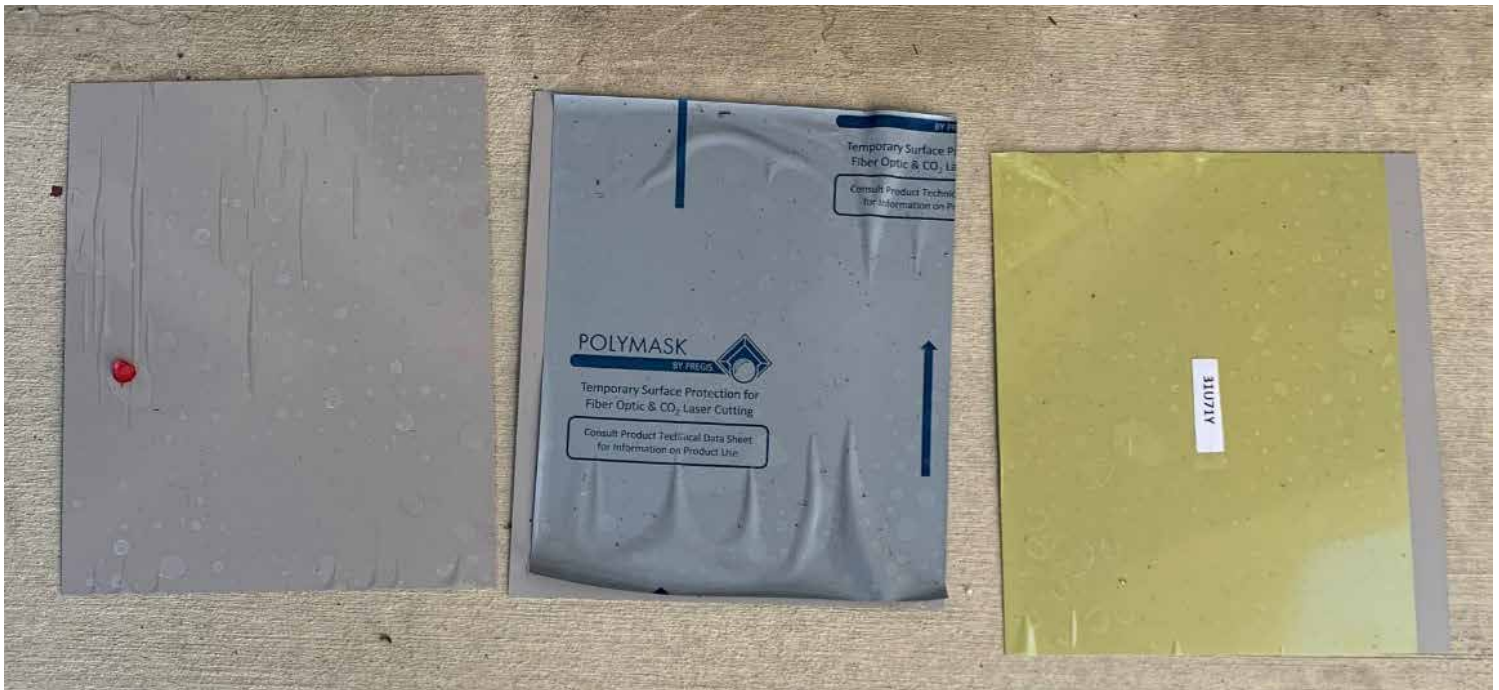
Product testing photo demonstrating mixed adhesion results for different strippable films
