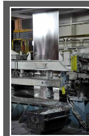
Application of the Metallic Coating at Steelscape Kalama
